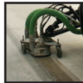
CURING COMPOUND REMOVAL
