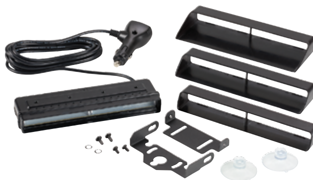
Each model includes light head, two suction cups, bail and pivot brackets, mounting hardware and three different length snap-on flash guards.
