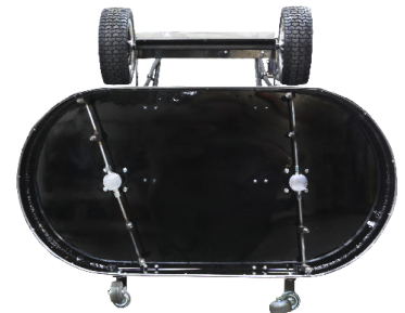
UNDERNEATH: SHOWING 4 NOZZLES PER ARM
