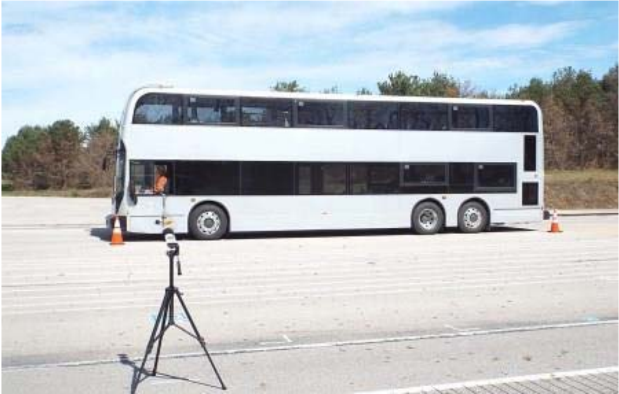
TEST BUS UNDERGOING EXTERIOR NOISE TESTING
