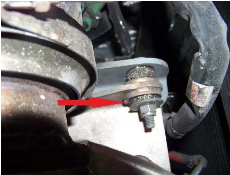
WORN EXHAUST MOUNT BUSHING (8,756 TEST MILES)
