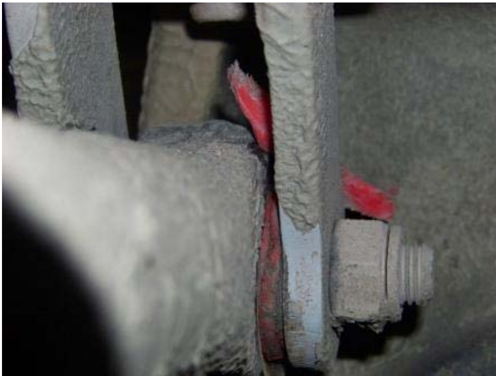
WORN FRONT SWAY BAR LINK BUSHING (7,399 TEST MILES)
