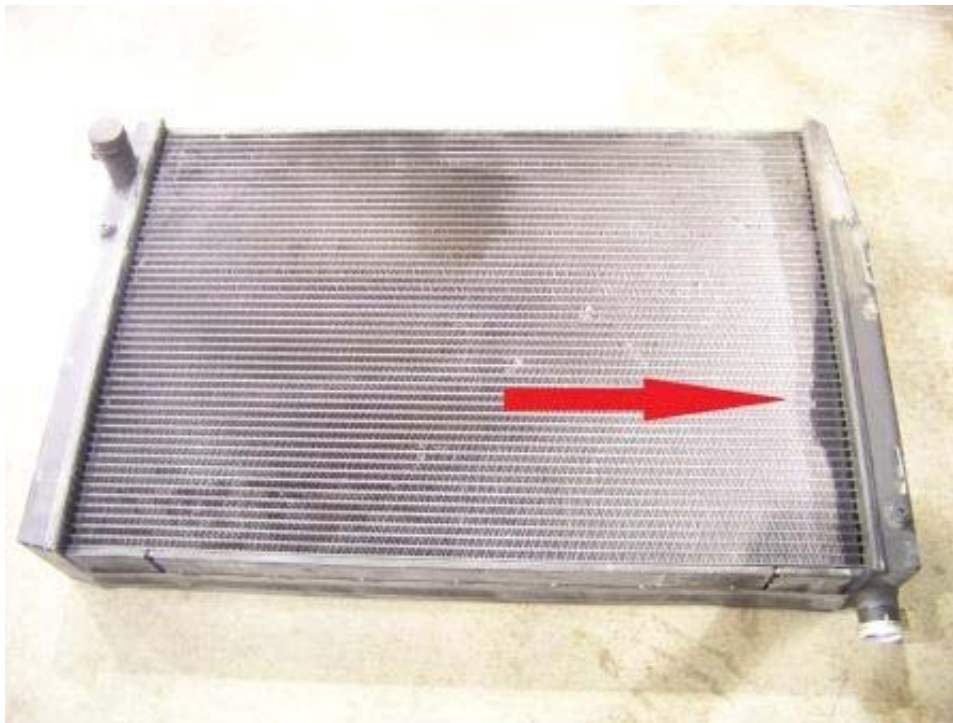
SPLIT RADIATOR (10,879 TEST MILES)
