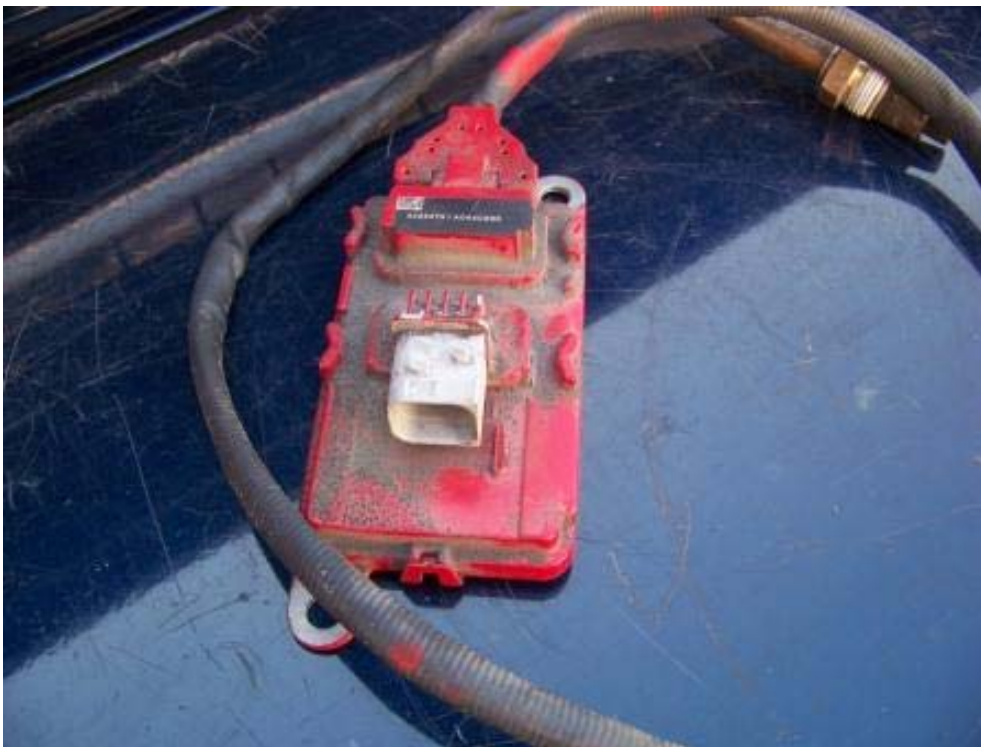
FAILED NOx SENSOR (12,244 TEST MILES)
