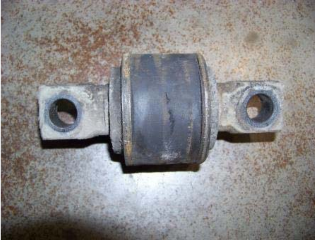
WORN RADIUS ROD BUSHING (8,756 TEST MILES)
