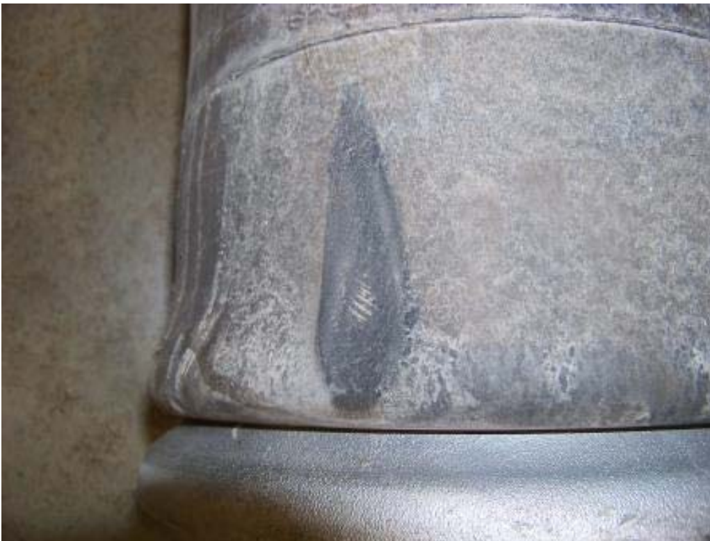
LEAKING LEFT FRONT AIR BAG (6,312 TEST MILES)
