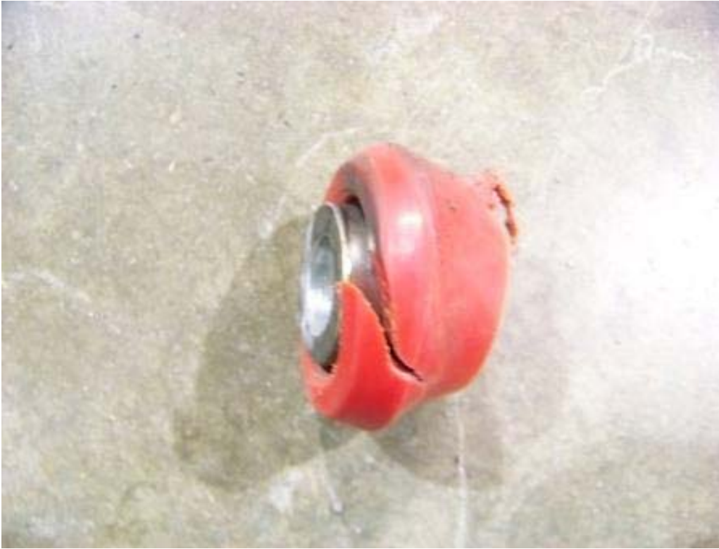
WORN RIGHT FRONT SWAY BAR BUSHING (6,120 TEST MILES)
