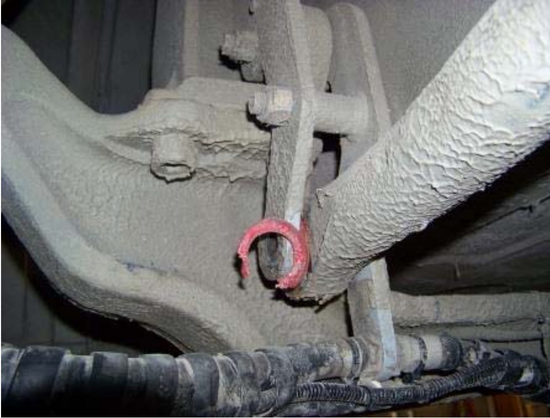
WORN FRONT SWAY BAR BUSHING (8,756 TEST MILES)
