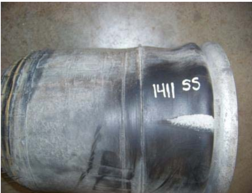
WORN AIR BAG FROM CONTACT WITH SHOCK (10,231 TEST MILES)
