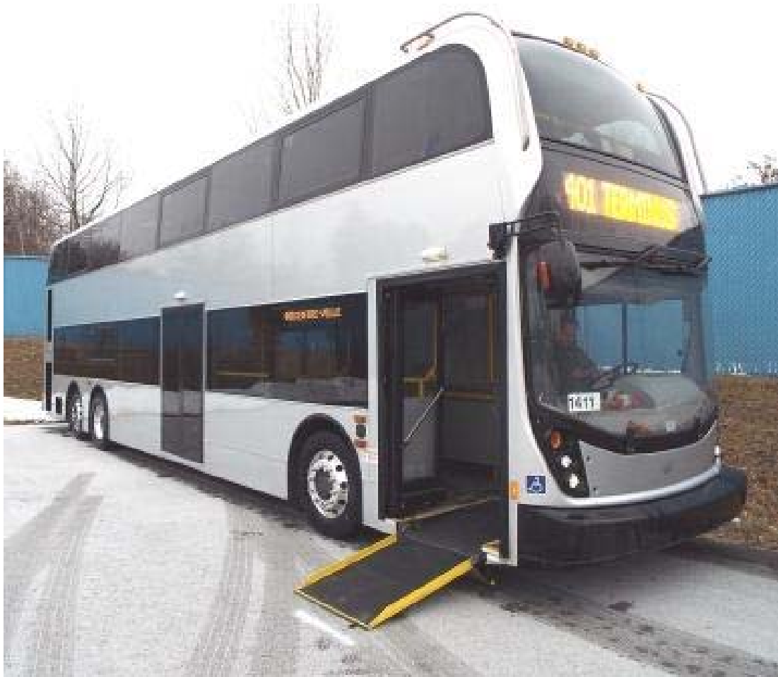
ALEXANDER DENNIS MODEL E500 EQUIPPED WITH A RICON MODEL R16215A HANDICAP RAMP
