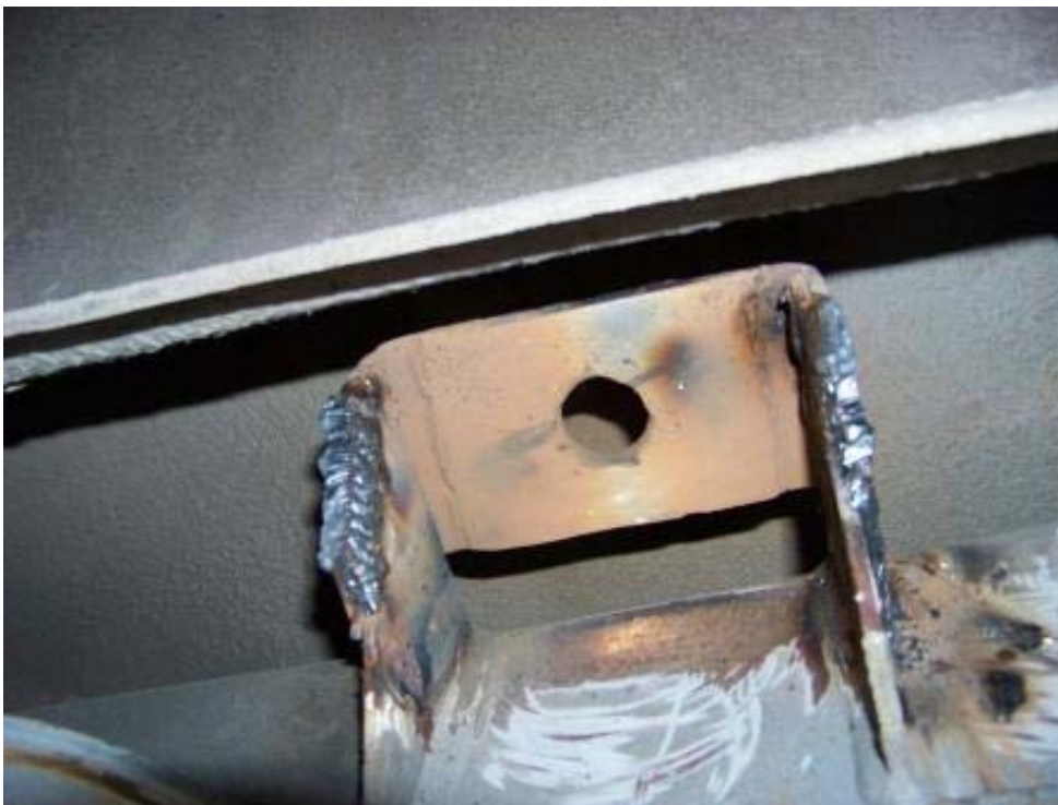
BROKEN UPPER SHOCK MOUNT (14,239 TEST MILES)
