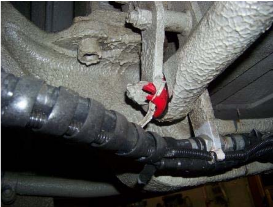
FRONT SWAY BAR BUSHINGS ARE WORN (4,869 TEST MILES)
