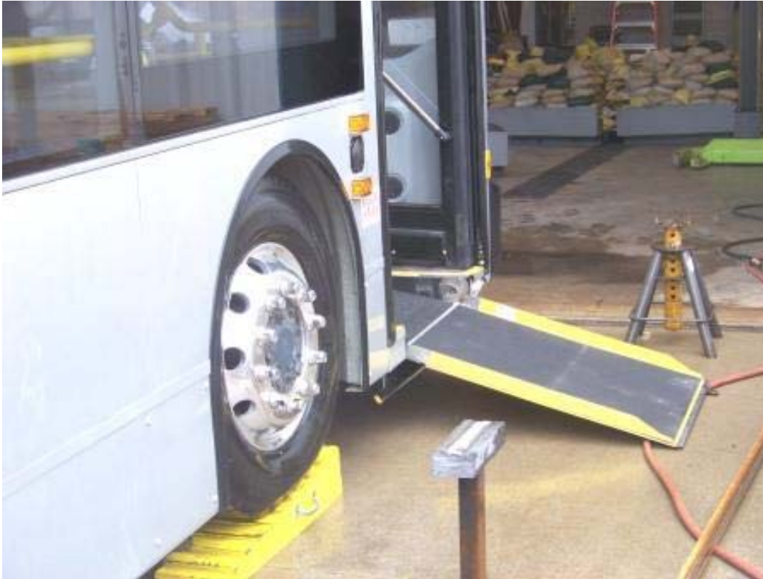
RIGHT FRONT WHEEL SIX INCHES HIGHER
