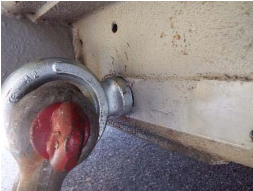
DEFORMATION OF LEFT TOW EYE
