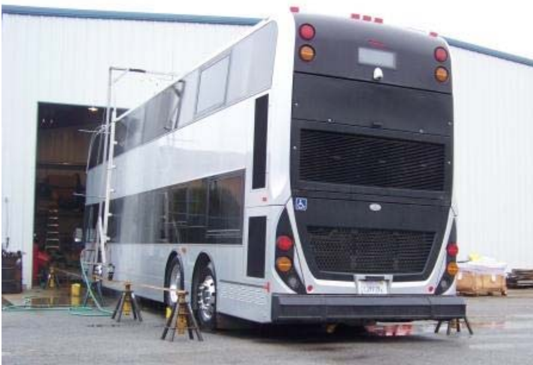
LEFT TAG WHEEL SIX INCHES LOWER
