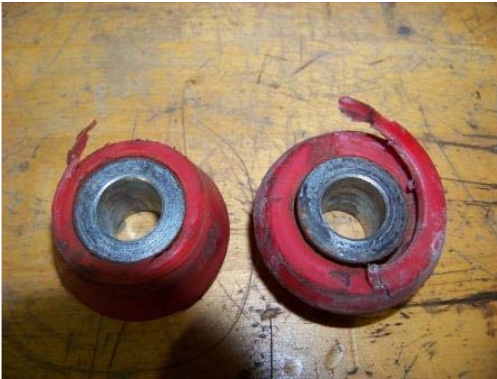
WORN FRONT SWAY BAR BUSHINGS (11,117 TEST MILES)
