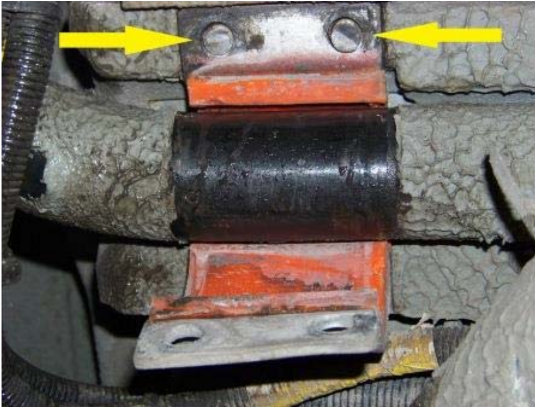
FRONT SWAY BAR; BROKEN CLAMP BOLTS (10,231 TEST MILES)
