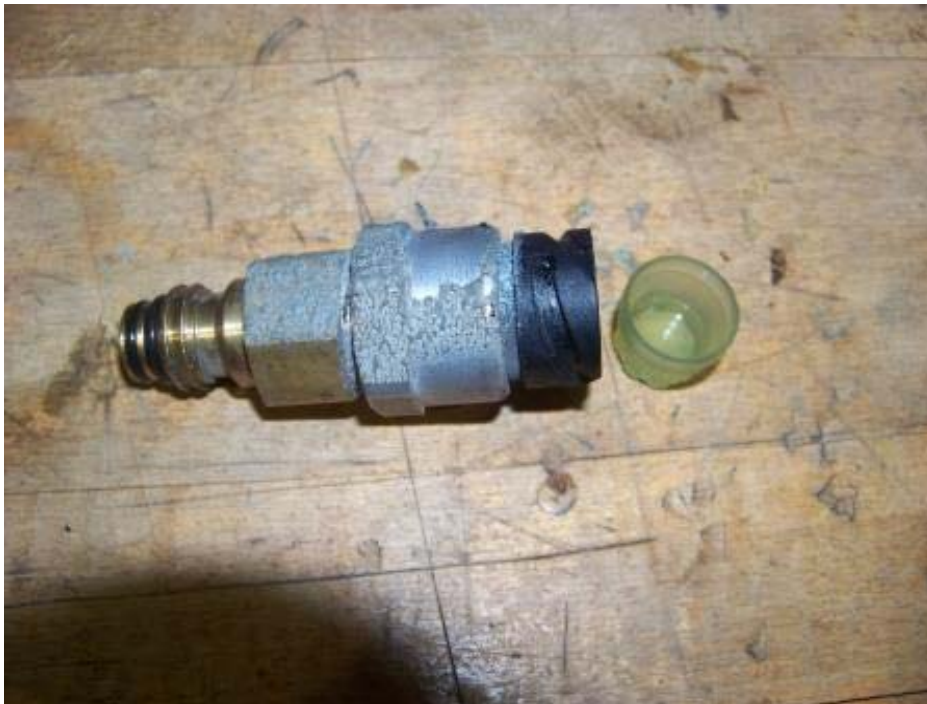
LEAKING AIR PRESSURE SENSOR (8,756 TEST MILES)
