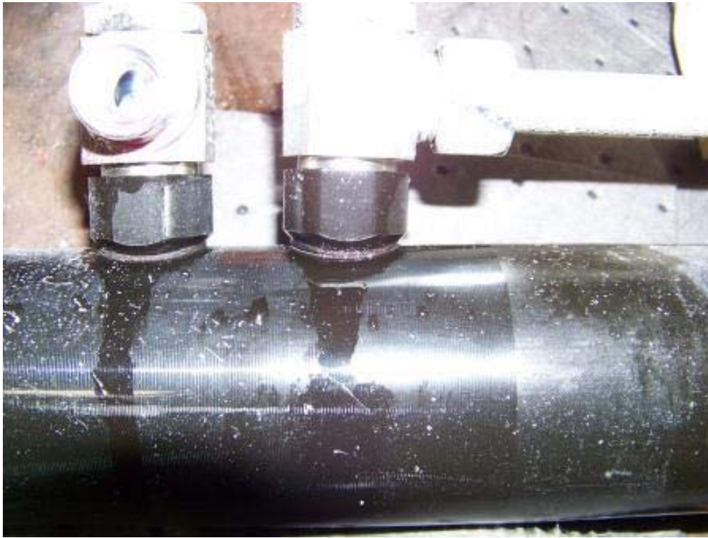
CRACKED PORTS ON THE TAG AXLE CENTERING CYLINDER (6,312 TEST MILES)
