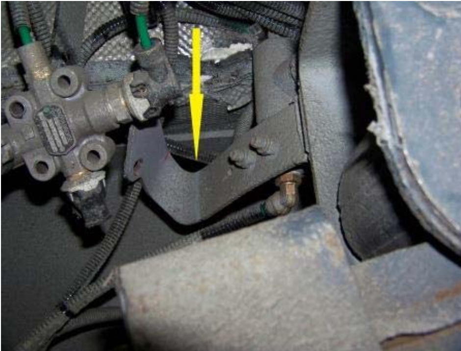
BENT LEVELING VALVE MOUNT (1,281 TEST MILES)
