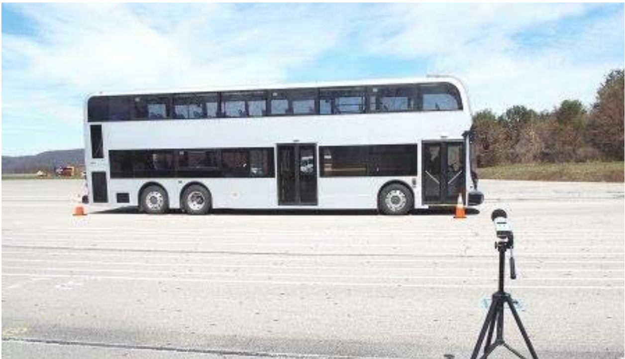
TEST BUS UNDERGOING EXTERIOR NOISE TESTING
