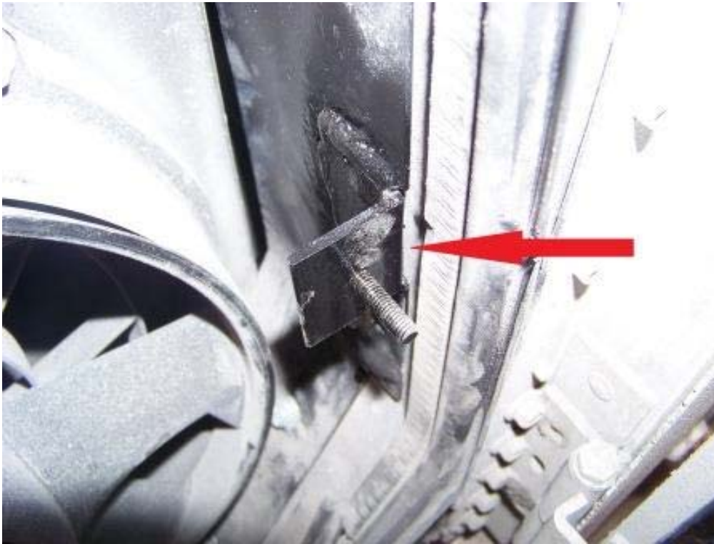
BROKEN ENGINE COOLING FAN BOX TAB (10,231 TEST MILES)
