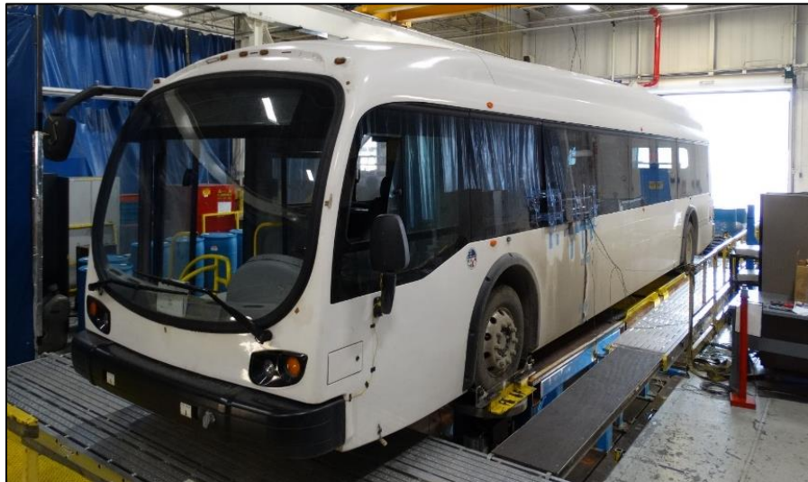
Figure 7-Catalyst 4-Post Durability Test
