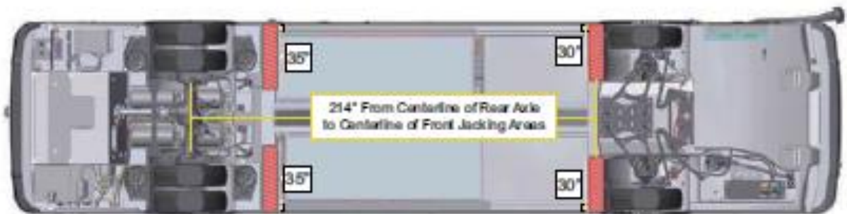
Figure 9-Proterra Recommended Lifting Zones
