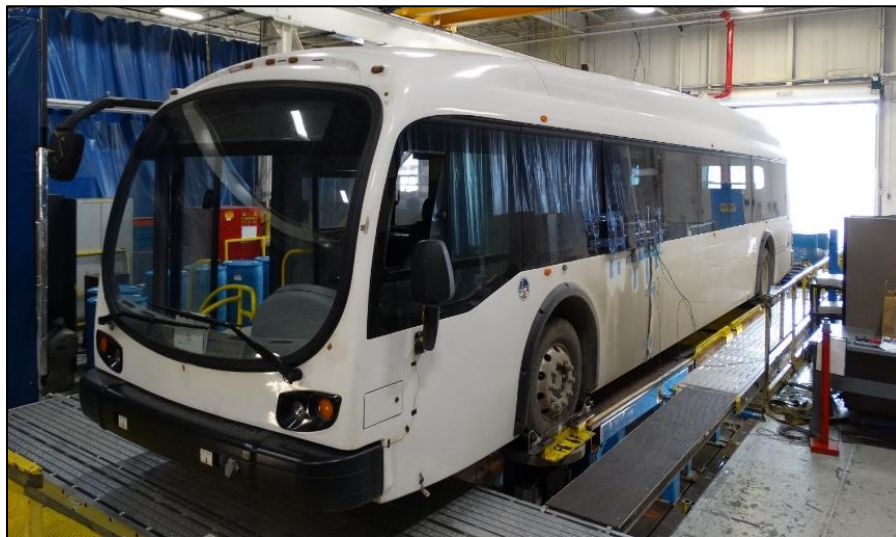
Figure 7-Catalyst 4-Post Durability Test
